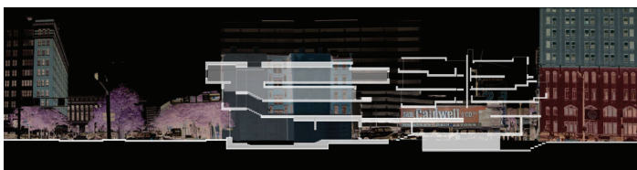
Figure 1. Students document precedent buildings in layers. This form of analysis enables them to study aspects of the buildings independently of other forces. Much is learned in the later synthesis when the layers are combined and interrelationships between compositional systems are made obvious. This image shows the cumulative information in the overlaid drawings.
